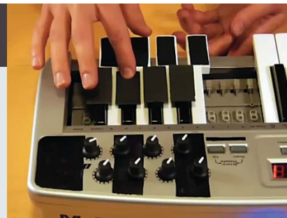
FIG. 1: Moldover ( moldover.com ) deconstructs M-Audio Oxygen 8 keyboards to put the controls where you want.
